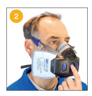
2. Lightly press the seal check button until you feel resistance. Hold the button in this position and inhale gently. If you feel the facepiece collapse slightly and pull closer to your face with no leaks between the face and facepiece, a proper seal has been obtained.
